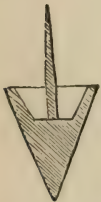
Fig. 32 represents a section through the axis of a cast-iron shoe and wrought-iron bolt for a pile.
